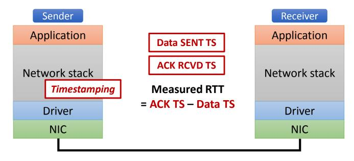
RTT measured from kernel gets affected by host delay jitter
