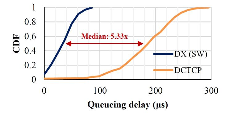
DX reduces median queuing delay by 5.33 times from DCTCP
