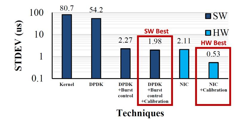
Accuracy of HW timestamping is sub-microsecond scale
